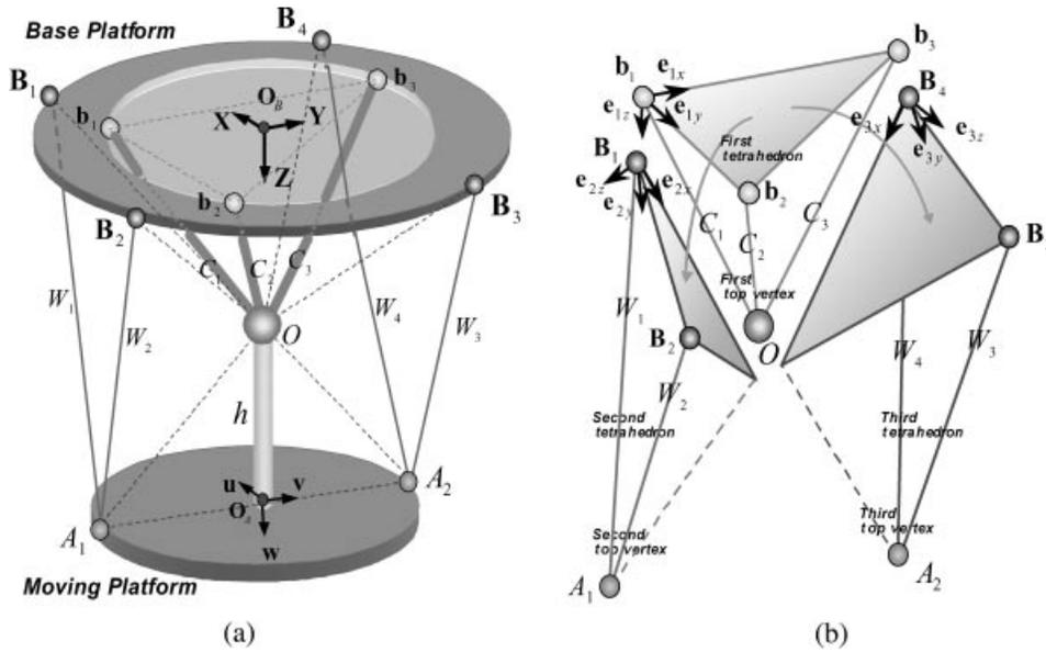
**Figure 6.** A 2-parallel mechanism with three cylinders and four wires, and tetrahedron configurations for its forward kinematics.
