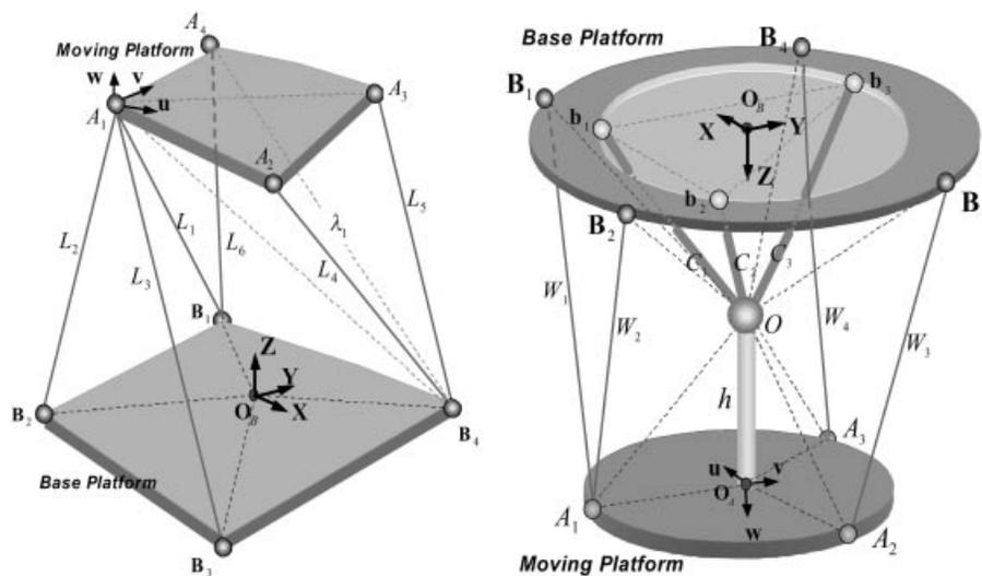
(c) A modified structure of the  $(3-1-1-1)^2$  parallel mechanism (d) A modified structure of the 2-2 parallel mechanism
