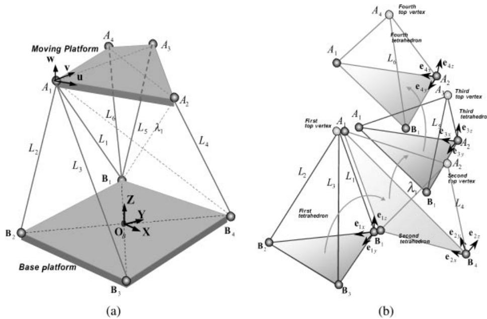
Figure 5. A  $(3-1-1-1)^2$  parallel mechanism and tetrahedron configurations for its forward kinematics.
