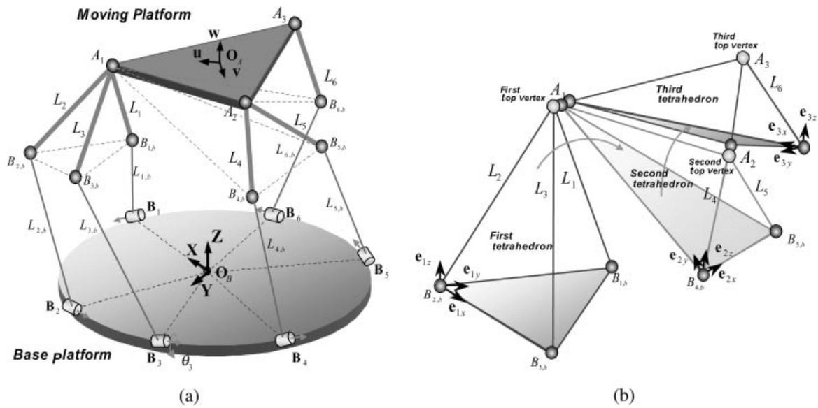
Figure 4. A 3-2-1 HEXA mechanism, and tetrahedron configurations for its forward kinematics.
