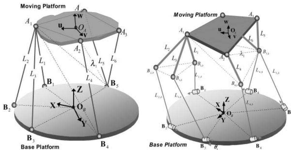
(a) A modified structure of the 3-2-1 parallel mechanism (b) A modified structure of the 3-2-1 HEXA mechanism
