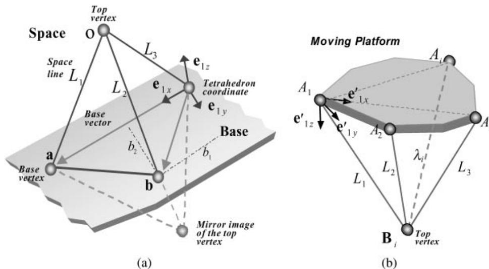
Figure 1. Kinematic modeling of a tetrahedron constructed on the parallel manipulator.
