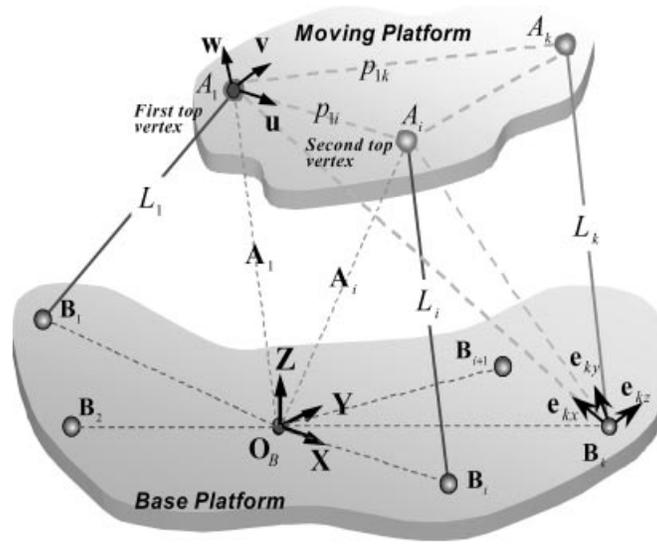
**Figure 2.** A parallel mechanism with two top vertices and another joint position on the moving platform with a known space line.
