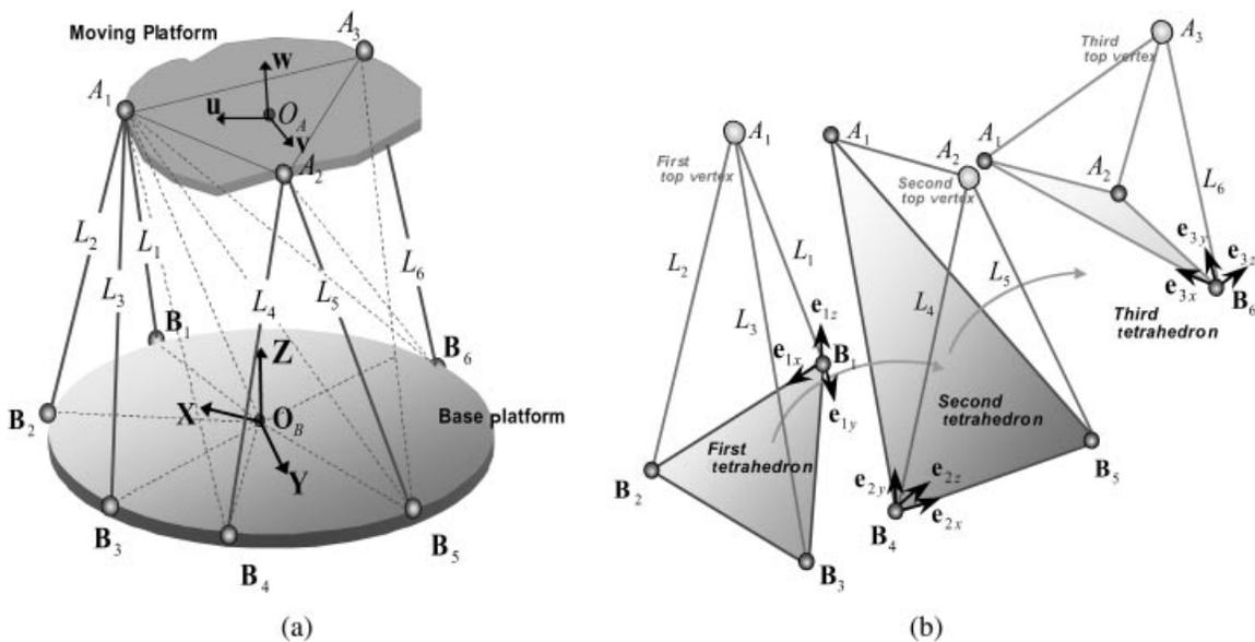
Figure 3. A 3-2-1 parallel mechanism, and tetrahedron configurations for its forward kinematics.
