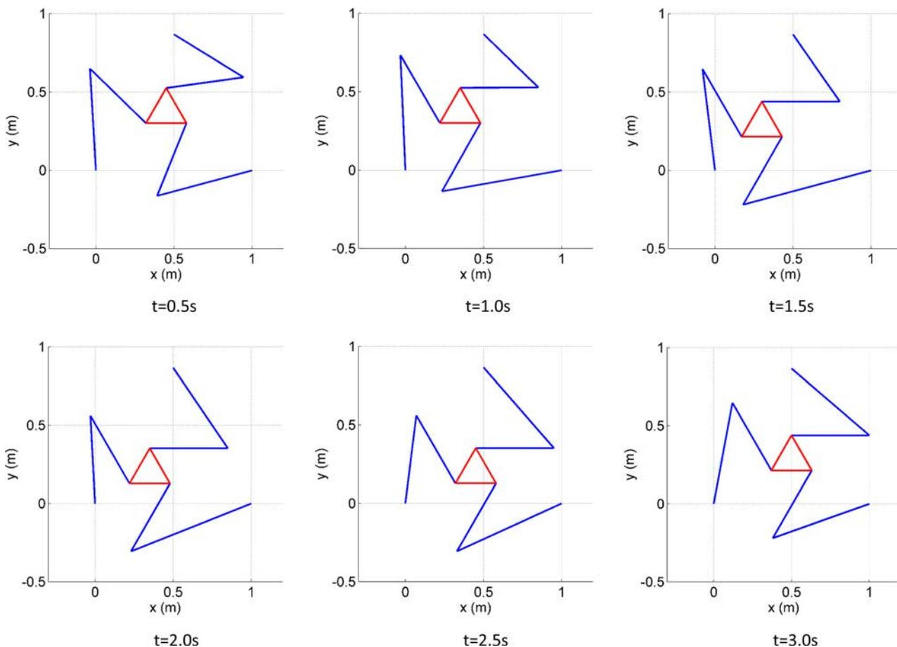
**Fig. 9 Joint configurations during the trajectory: case of optimized null-space solution**
