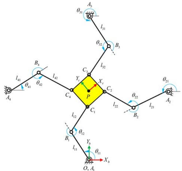
Fig. 4 Schematic diagram of the 4-RRR redundantly actuated manipulator
