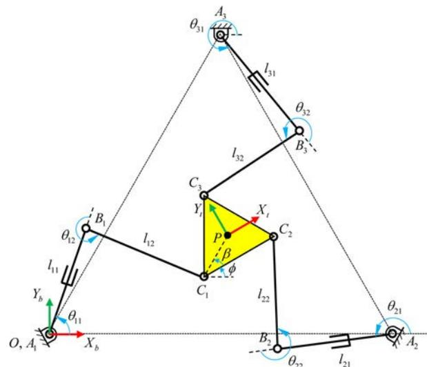
**Fig. 2 Schematic diagram of the 3-RPRR kinematically redundant manipulator**
