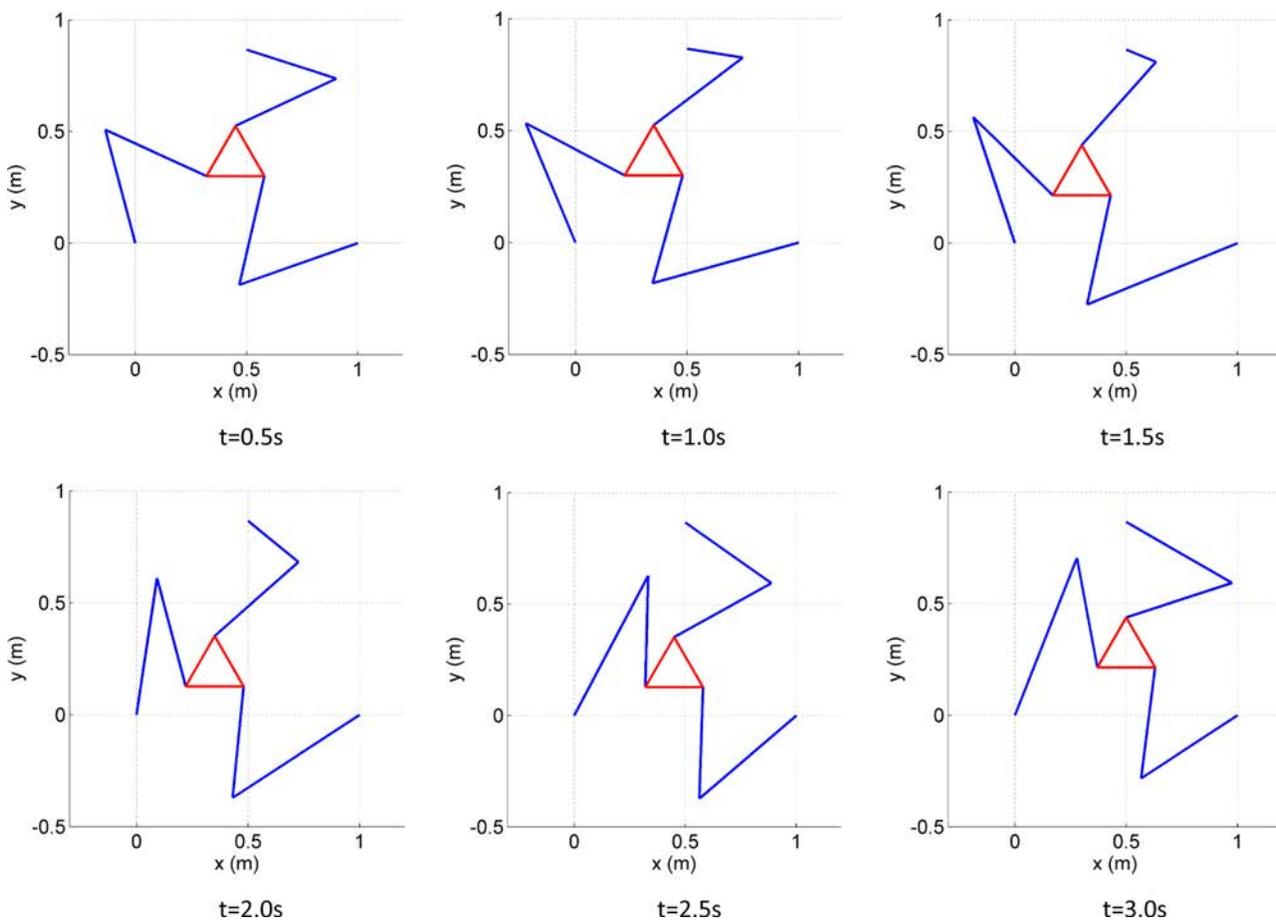
**Fig. 7 Joint configurations during the trajectory: case of minimum norm solution**
