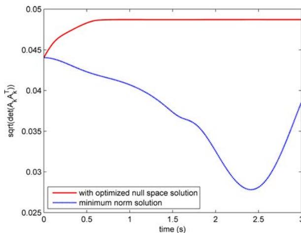
**Fig. 11 Variations of  $\sqrt{\det(AA^T)}$  for two different inverse kinematic solutions of 3-RPRR PM**
