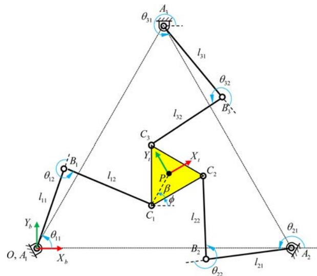
**Fig. 1 Schematic diagram of the 3-RRR nonredundant manipulator**
