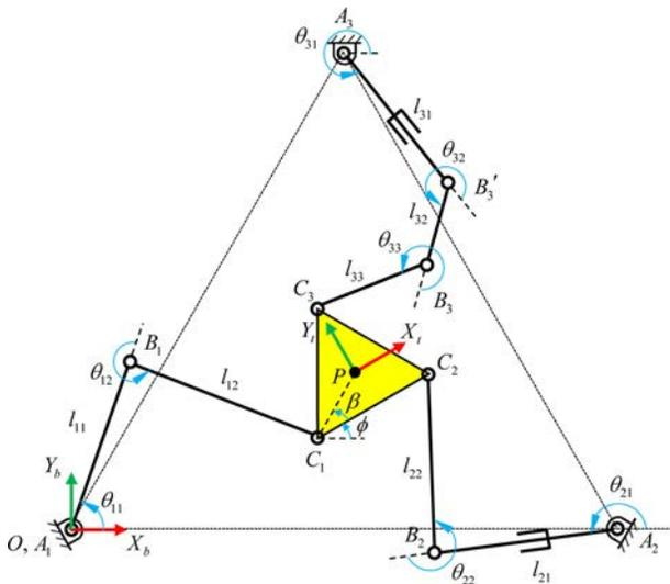
Fig. 3 Schematic diagram of the RRR-RPRR-RPRRR kinematically redundant manipulator
