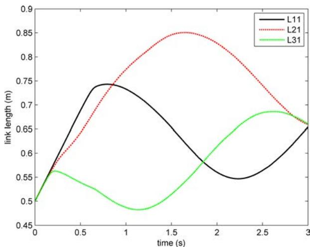
**Fig. 10 Link length variations of the three redundant prismatic joints: case of optimized null-space solution**
