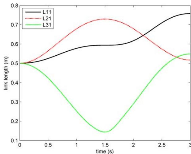
**Fig. 8 Link length variations of the three redundant prismatic joints: case of minimum norm solution**
