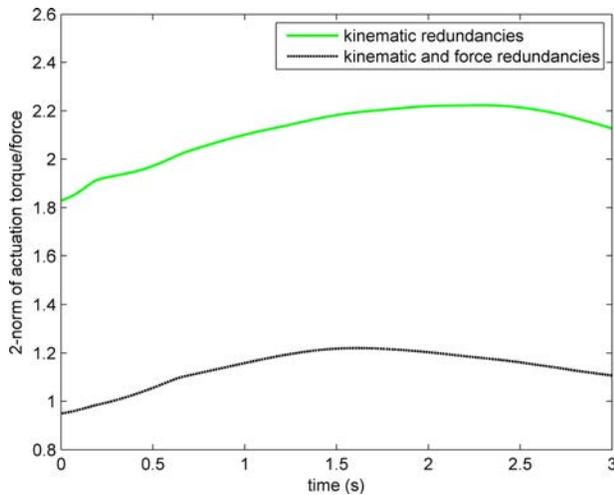
**Fig. 12 Comparison of 2-norm of the actuation torque/force of the 3-RPRR PM with that of the 3-RPRR PM**
