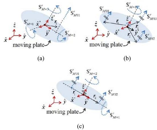
Fig. 10. Equivalent mechanism constraints for the  $2T_{x^*y^*}$ -type 2-DOF PM: (a) Type-A mechanism constraints; (b) type-B mechanism constraints; (c) type-C mechanism constraints.
