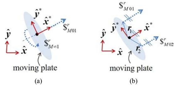
Fig. 8. Equivalent mechanism constraints for the  $1T_{y^*}$ -type 1-DOF PM: (a)  $F_{x^*}$ - and  $C_z$ -type constraints; (b) two  $F_{x^*}$ -type constraints.
