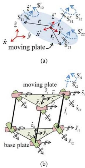
Fig. 12. Over-constrained PM: (a) Limb constraints; (b) spatial  $2T_{x^*y^*}$  parallelogram.
