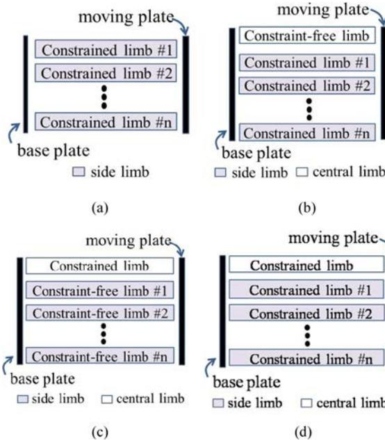
Fig. 7. PM structures: (a) With several side limbs; (b) with a constraint-free central limb and several constrained side limbs; (c) with a constrained central limb and several constraint-free side limbs; (d) with a constrained central limb and several constrained side limbs.
