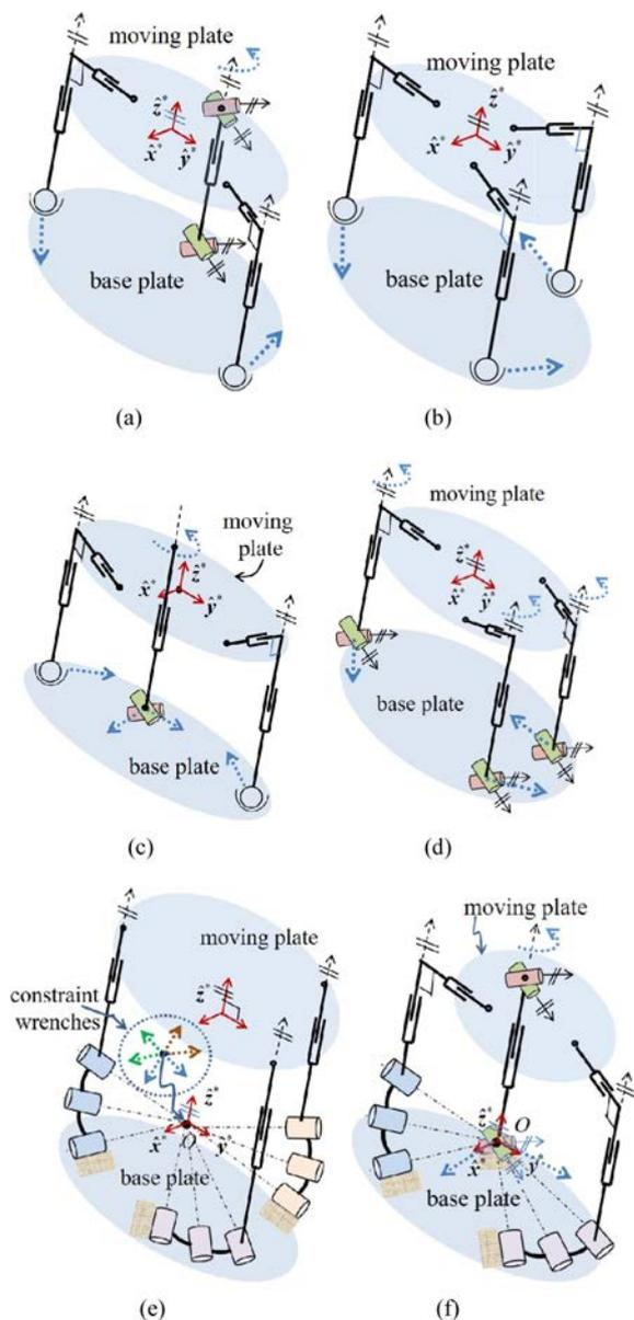
Fig. 14. The  $1T_{z^*}2R_{x^*y^*}$  type spatial 3-DOF PMs with three limbs: (a) With two  $F_{x^*}$ -limbs and one  $C_{z^*}$ -limb; (b) with three two  $F_{x^*}$ -limbs; (c) with two  $F_{x^*}$ -limbs and one  $F_{x^*y^*}C_{z^*}$ -limb; (d) with three  $F_{x^*}C_{z^*}$ -limbs; (e) with three  $F_{x^*y^*}$ -limb; (f) other version of PM in (a) with the same base point of all three limbs.
