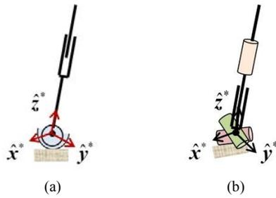
Fig. 5. The admissible joint structures of the  $F_{x^*y^*}C_{z^*}$ -limb: (a)  $(R_{x^*}, R_{y^*}, R_{z^*})_O P_{z^*}$  type limb; (b)  $(R_{x^*}, R_{y^*})_O P_{z^*} (R_{z^*})_O$  type limb.
