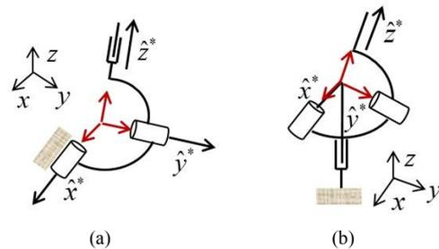
Fig. 6. The  $F_{x^*y^*}C_{z^*}$ -limb and the  $F_{xy}C_{z^*}$ -limb: (a) The  $(R_{x^*y^*}, R_{y^*k^*}, R_{k^*y^*})_O P_{z^*}$  type limb; (b)  $P_z (R_{x^*y^*}, R_{y^*k^*})_O$  type limb.
