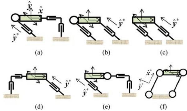
Fig. 9. Planar  $1T_{y^*}$ -type 1-DOF PMs with two constrained limbs: (a) ( $\{\hat{S}_{L01}^r\}, \{\hat{S}_{L01}^r\}$ ); (b) ( $\{\hat{S}_{L01}^r\}, \{\hat{S}_{L01}^r, \hat{S}_{L01}^r\}$ ); (c) ( $\{\hat{S}_{L01}^r, \hat{S}_{L01}^r\}, \{\hat{S}_{L01}^r, \hat{S}_{L01}^r\}$ ); (d) ( $\{\hat{S}_{L01}^r\}, \{\hat{S}_{L01}^r, \hat{S}_{L01}^r\}$ ); (e) ( $\{\hat{S}_{L01}^r, \hat{S}_{L01}^r\}, \{\emptyset\}$ ); (f) ( $\{\hat{S}_{L01}^r\}, \{\hat{S}_{L01}^r\}$ ).
