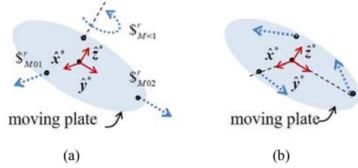
Fig. 13. Equivalent mechanism constraints for the  $1T_{z^*}2R_{x^*y^*}$ -type spatial 3-DOF PM: (a) Mechanism constraints; (b) equivalent mechanism constraints.
