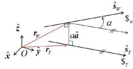
Fig. 1. Geometry of two screw axes.
