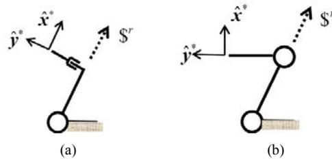
Fig. 3. Admissible joint structures of the planar  $F_{x^*}$ -type limb: (a)  $R_{zLx^*}P_{x^*}$ -type limb; (b)  $R_{zLx^*}R_{zLx^*}$ -type limb.
