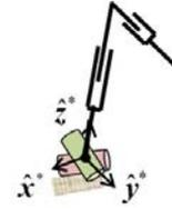
Fig. 4. The admissible joint structures of the  $F_{x^*}C_{z^*}$ -limb:  $R_{x^*Iz^*}R_{y^*Iz^*}P_{z^*}P_{y^*}$  type limb.
