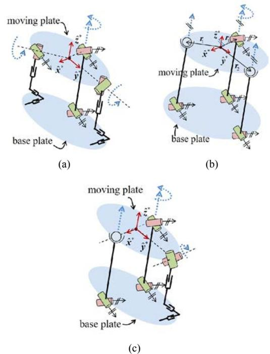
Fig. 11. Examples of the  $2T_{x^*y^*}$ -type 2-DOF asymmetric and non-over-constrained PMs: (a) With type-A mechanism constraints; (b) with type-B mechanism constraints; (c) with type-C mechanism constraints.
