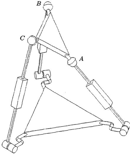
Figure 3: An RO-type singularity of a 3-RPS mechanism
