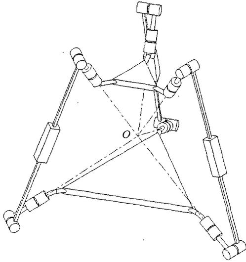
**Figure 2:** A 3-*UPU* wrist in a constraint singularity
