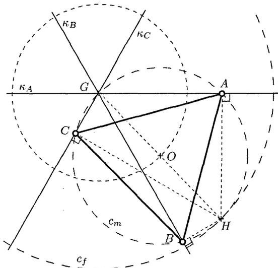
Figure 5: Constraint singularities of a 3-RPS mechanism
