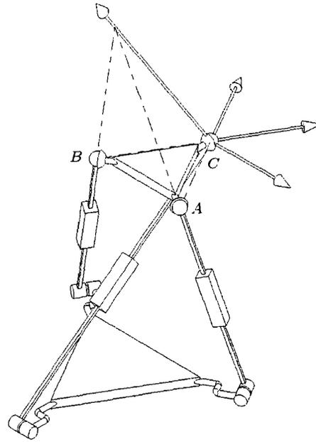
Figure 4: A constraint singularity of a 3-RPS mechanism
