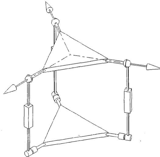
Figure 6: A 3-RPS PM in a constraint singularity
